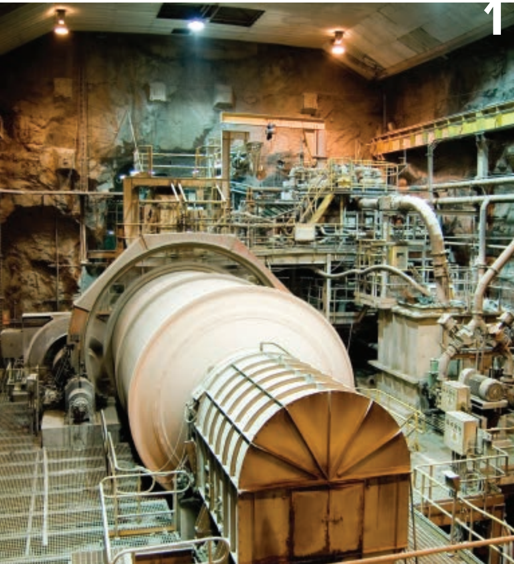
1. A 20-foot diameter ball mill rotates at a copper mine's underground processing facility in Chile. This process breaks copper-bearing ore from golf-ball sized pieces into dust. 2. Froth 3. Only a very small percentage of copper is removed from tons of ore dug out of this Chilean copper mine, the world's largest open-pit mine. The overburden, or leftover slag, is a heavy sludge that is disposed of in enormous man-made mountains. 4. Melted copper. 5. Copper cathode in electrolysis. 6. Thousands of sheets of copper are grown in an enormous acid bath at a mining processing facility in Chile.
